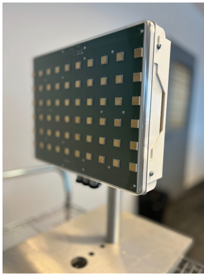
Figure 6. mMIMO O-RAN radio whitebox
