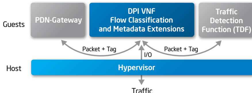
Figure 3. DPI Implemented as a Virtual Network Function
