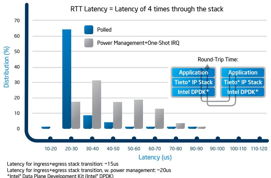
**Figure 6.** Latency distribution of GTP-U traffic when testing 1) without power management in a purely polled setup and 2) in a setup with power management and the one-shot interrupt feature (based on an Intel® Xeon® Processor E5-2600 @ 3.4GHz).
